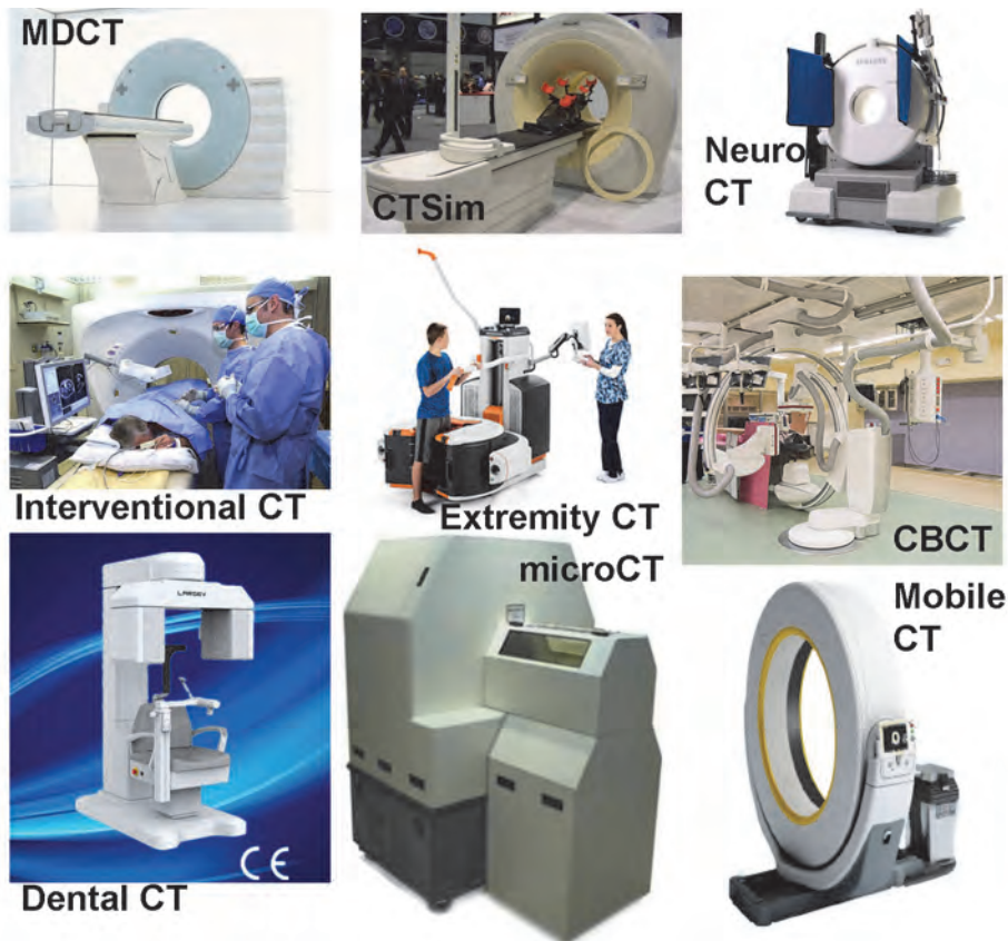
Figure 1.18 Examples of CT scanning “flavors” from a variety of practice settings. All of these scanners use x-ray projection data acquired from a plurality of angles about an object to reconstruct tomographic images.
