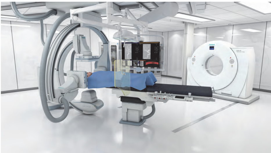
Figure 1.13 It is not uncommon to find different flavors of CT used in the same environment. This image shows the combination of an interventional CBCT system coupled with an “MDCT on rails.” Notice the metal strips on the floor in front of the MDCT scanner. Those strips are guides allowing the MDCT scanner to move over the patient, enabling volumetric image acquisition where the patient remains stationary, and the scanner translates over them. (Image provided by Siemens Healthcare.)
