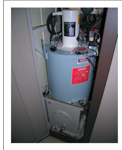
Figure 9.17 A klystron inside the gantry stand of a high-energy standing wave linac. The tank of insulating oil can be seen at the bottom.
