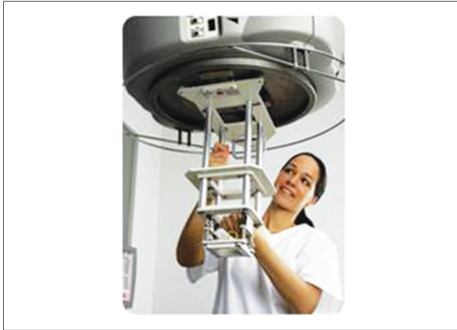
Figure 9.23 A therapist prepares to attach an electron applicator to the collimator of a linac. The applicator provides extra collimation. (Courtesy of Elekta AB.)
